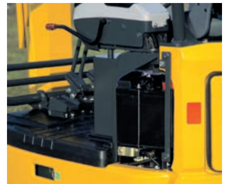
Left bonnet: easy access to the battery
