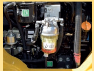
Large fuel filter and fuel pre-filter with water separator protect the engine
