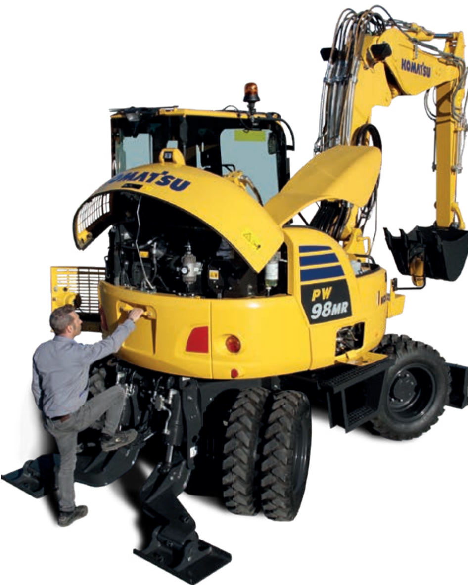
All major maintenance points can be easily reached from ground level
